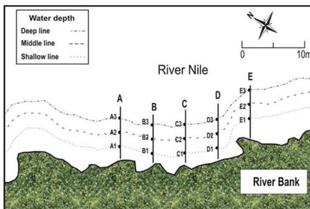
**Fig. 2:** A contour map of the studied site at the western bank of the River Nile showing the sampling plan.
